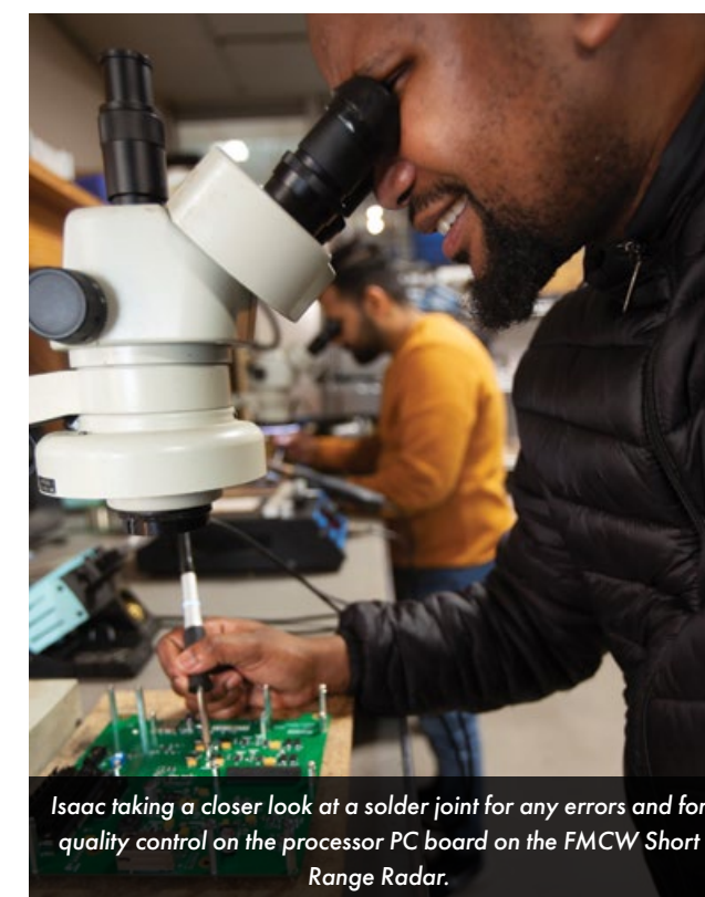
Isaac Mpheng, Graduate Designer: RF & Microwave, visually inspecting processor PC board on the FMCW Short Range Radar.
