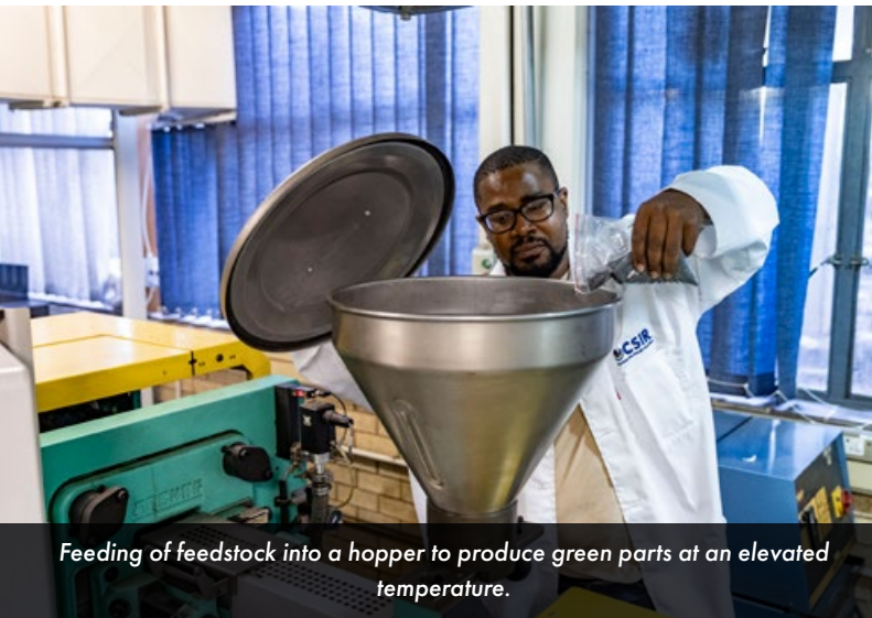
Mandy N Madigoe, Senior Engineer and Technical Leader for metal injection moulding (MIM) project, preparing an Arburg MIM machine to produce green components.
