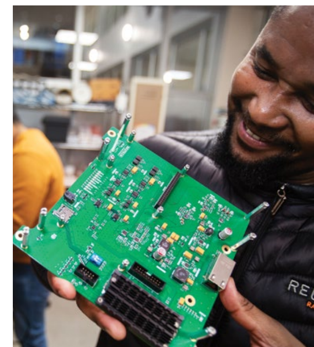
Isaac Mpheng, Graduate Designer: RF & Microwave, visually inspecting processor PC board on the FMCW Short Range Radar.
