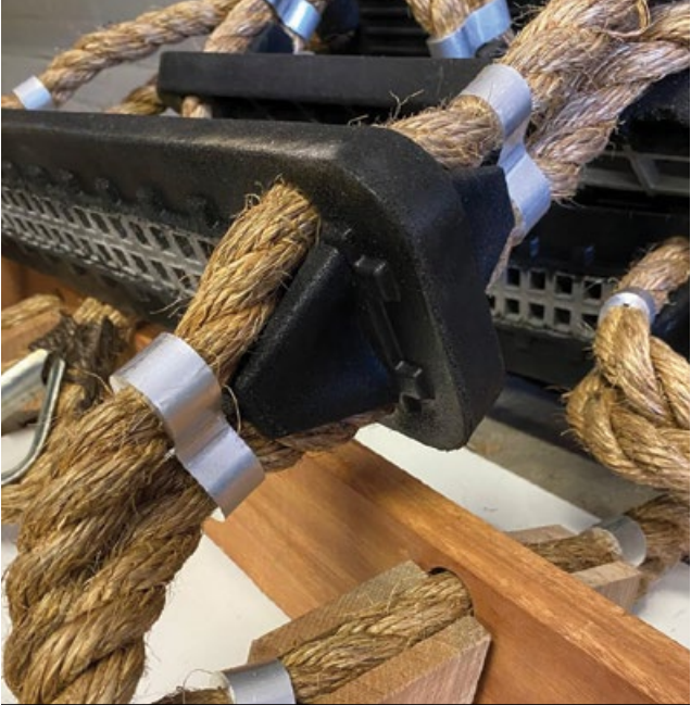
Whilst conventional pilot ladders make use of the tread and four poppets as separate components, a simplified assembly process has been developed that means the Sure Step is integrated into one single component. The product is also designed to make use of aluminium crimps for tying the treads in place as opposed to older ladders that would be tied together using twine.
