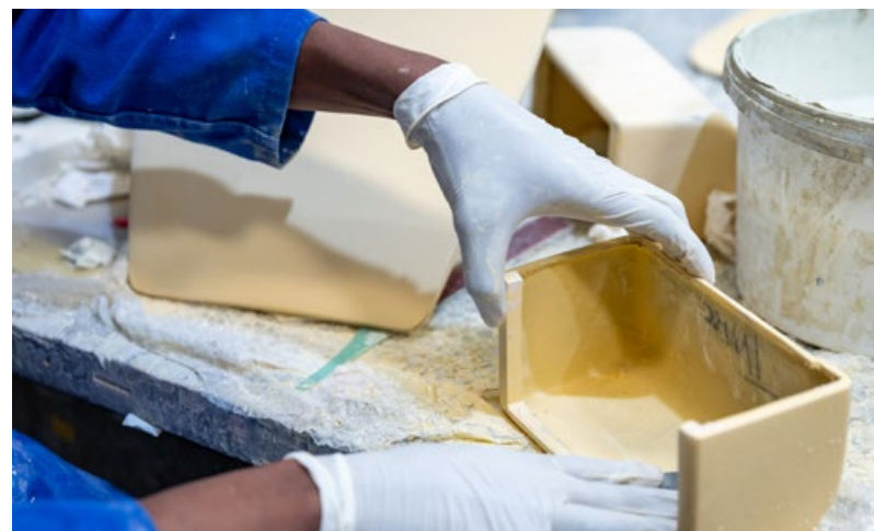
Components are manufactured from glass, Kevlar, and carbon fibre materials, utilising both traditional and advanced technologies such as the use of pre-impregnated fibres and resin-transfer manufacturing.
