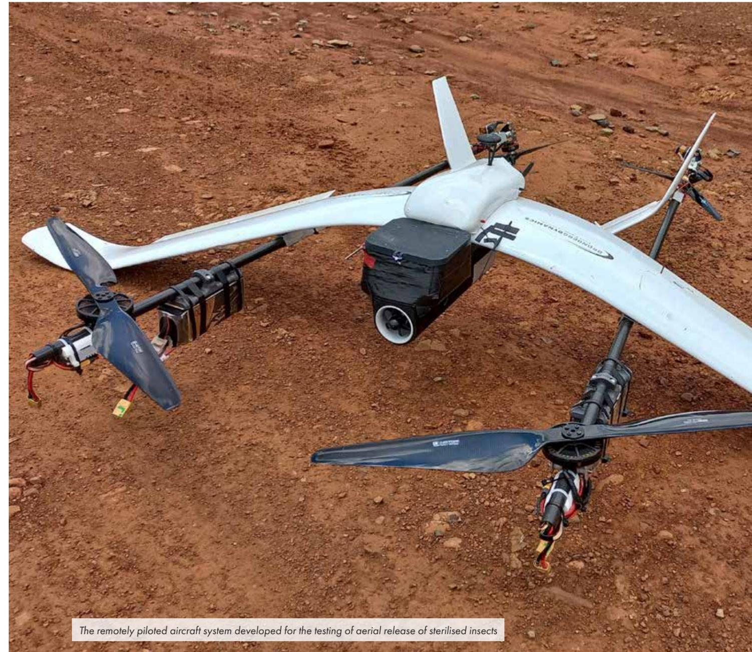
The remotely piloted aircraft system developed for the testing of aerial release of sterilised insects
