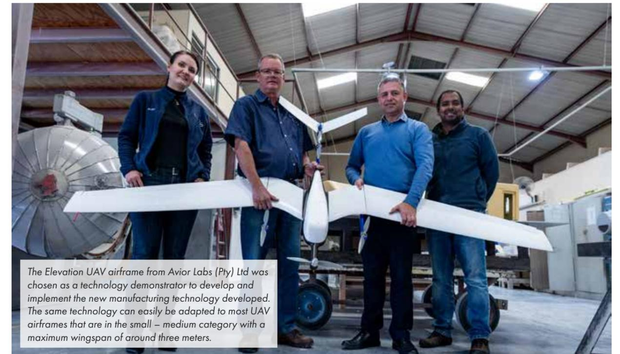
The Elevation UAV airframe from Avior Labs (Pty) Ltd was chosen as a technology demonstrator to develop and implement the new manufacturing technology developed. The same technology can easily be adapted to most UAV airframes that are in the small – medium category with a maximum wingspan of around three meters.
