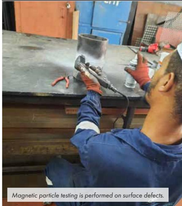
Magnetic particle testing is performed on surface defects.
