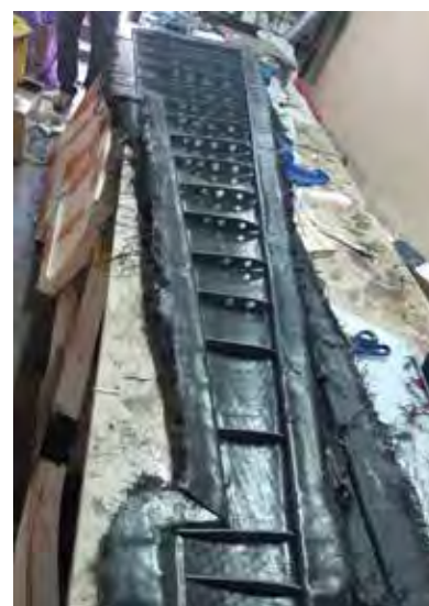
Carbon fibre wing skin with internal structure/ribs temporarily placed in position
