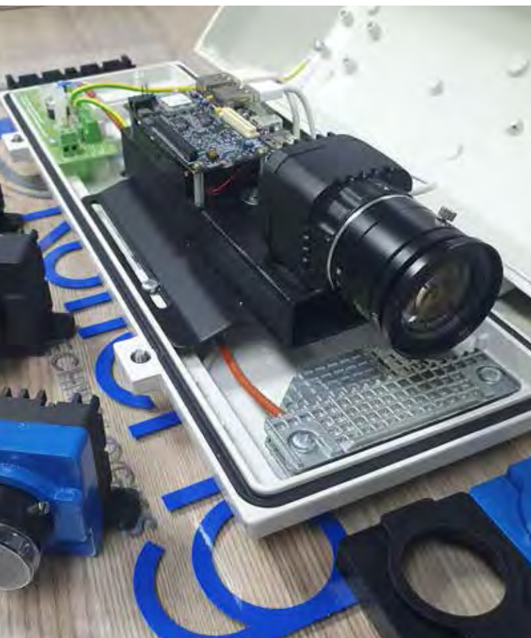
Jenasi SmartCAM enclosure with external Field Programmable Gate Array, System on Module
