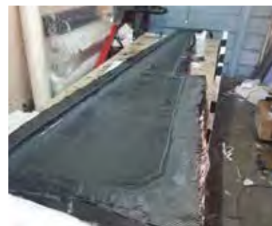
Carbon fibre wing skin layup after curing and before trimming
