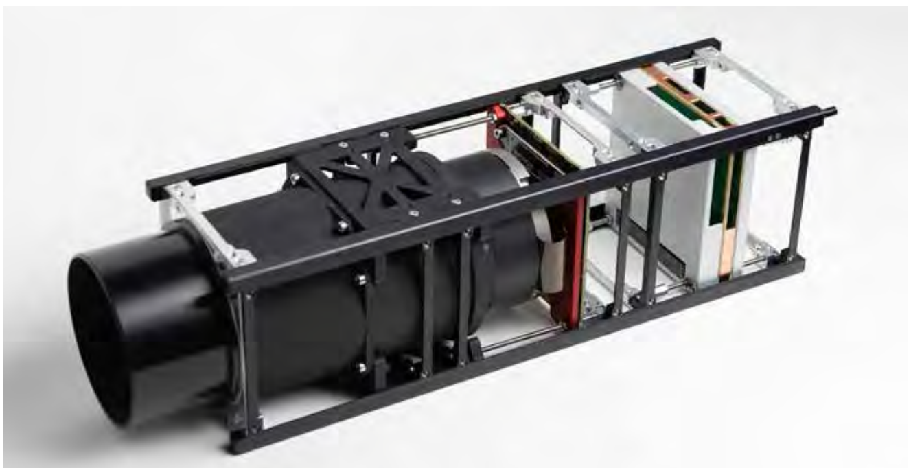
Nano-satellite space imager with the enclosure for the power control unit
