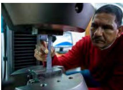
Static test of test piece produced by additive manufacturing
