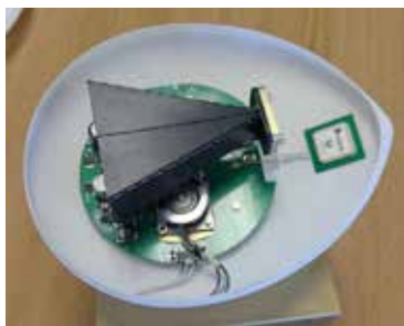
The airborne directional antenna with the lid removed. The horn antenna, printed circuit board with motor drive and GPS antenna can be seen.
