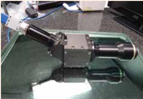
Figure 2: Hyperspectral imager prototype during testing
