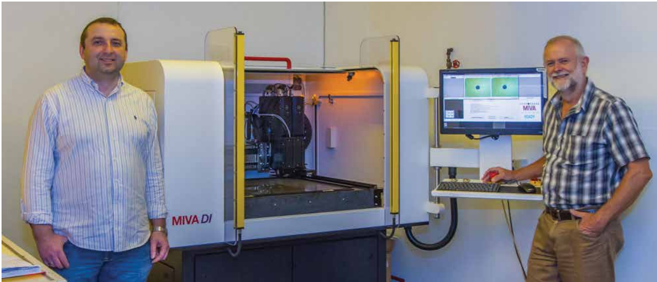
Figure 2: Direct Imaging equipment used for SKA PC Board Development
