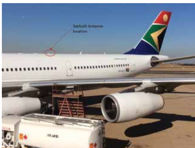
Figure 5: Location of SatAuth antenna on ZS-SLF aircraft
