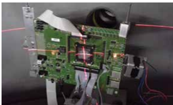
Figure 3: Experimental setup for radiation screening, beam alignment
