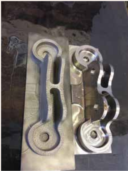
Figure 2: Engine brackets comparison: AM built from 304 Stainless steel (left) and machined from 17-4PH Stainless steel (right)
