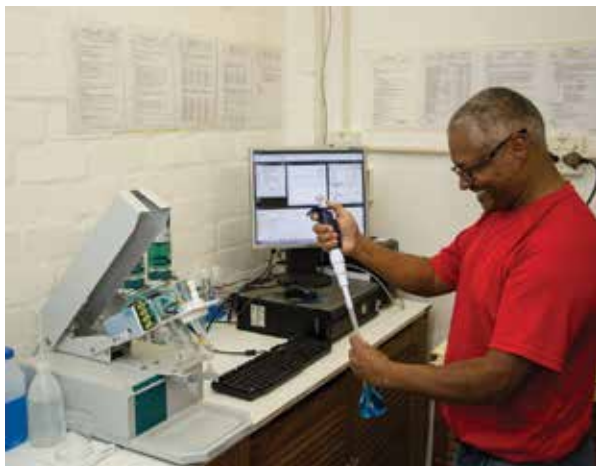
Figure 3: Cyclic Voltammetric Stripping (CVS) analysis equipment to analyse the reverse pulse plating chemistry
