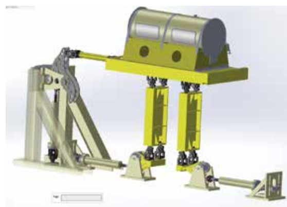
Figure 4: CAD model of sloshing apparatus at the UP
