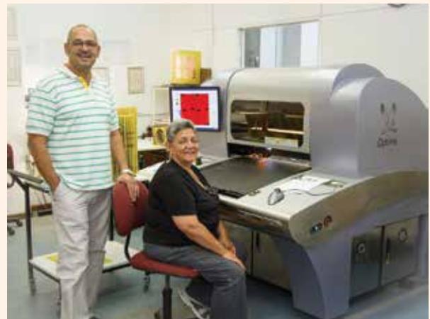
Figure 1: TraX staff working on the Camtek AOI machine used for SKA PC board development
