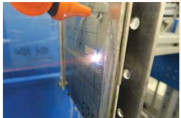
Figure 1: Working LSP cell (laser and optical system)
