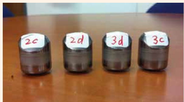
Figure 4: Laser peened tungsten carbide components
