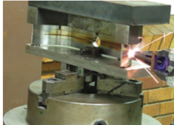
Figure 5: Laser welding of stainless steel gimbal beams
