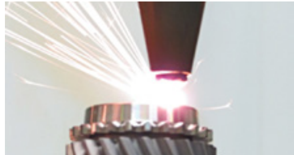
Figure 2: Laser beam welding of gear assembly
