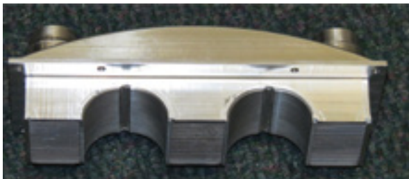
Figure 4: Laser welded heat exchanger assembly
