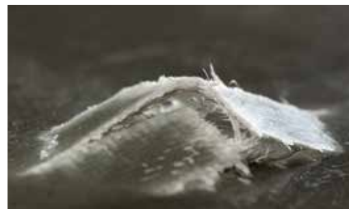
Induced impact damage
