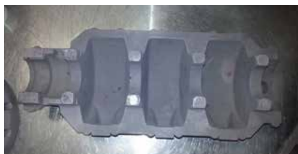
Aluminium casting showing isolated bleed-out of dye penetrant test
