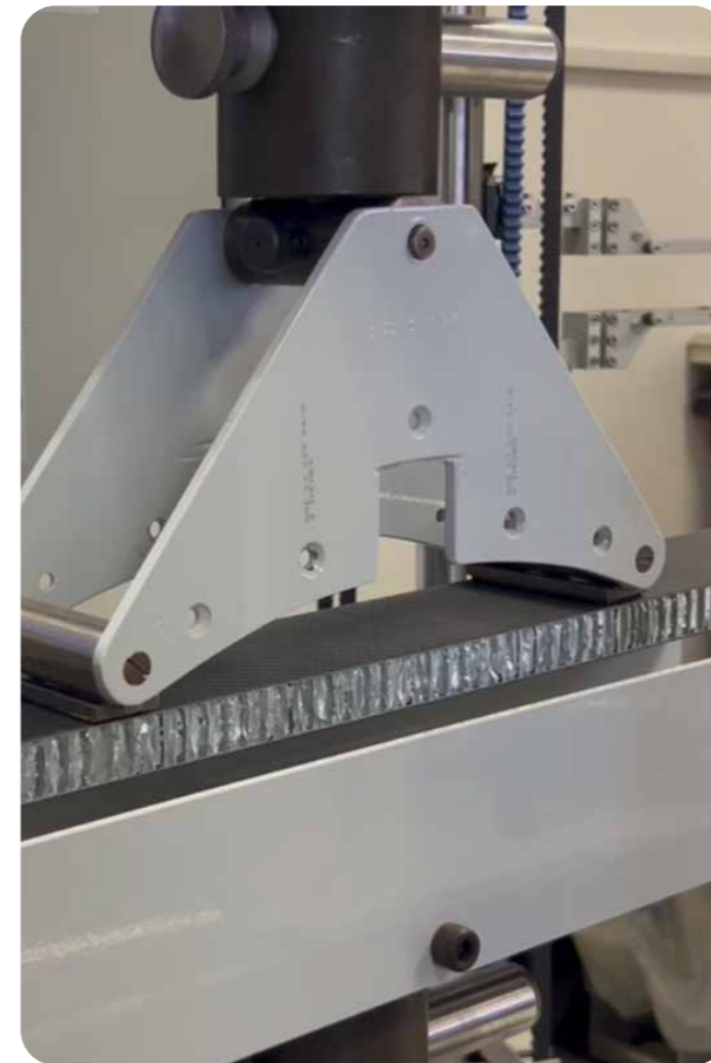
The test sample and setup for the long beam bending test to determine the bending stresses that the panel can withstand the core ribbons directions in the transverse and longitudinal direction. The tensile machine was used to compress the panel to cause it to bend and from which we could correlate our analytical results.
