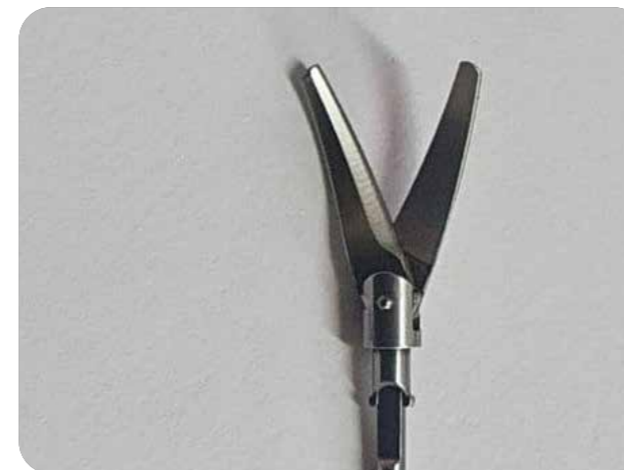
The front jaws are joined to the pull rod using laser welding and will then be inserted into the outer tube
