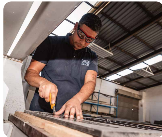
CNC machine operator, Fabian Kinnear, cutting the locating tabs to be able to remove the CNC cut components from the sheet of virgin HDPE
