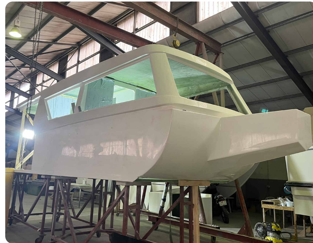
Front view of the first cabin produced from the mould
