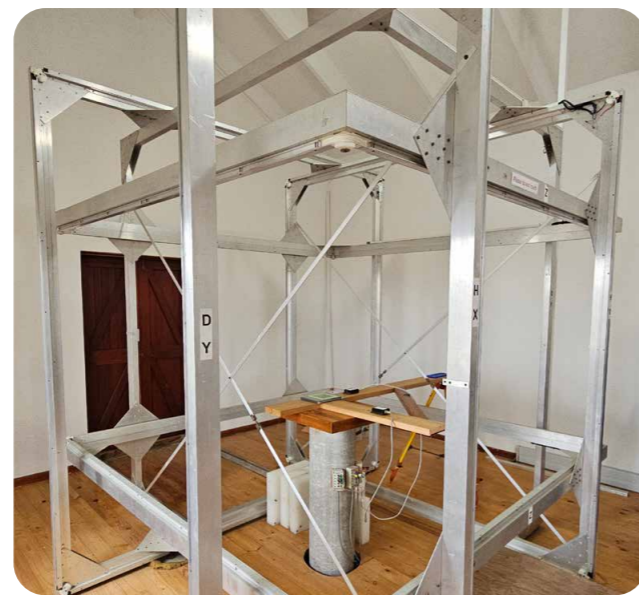
GNSS antenna dielectric material undergoing magnetic evaluation at SANSA’s tri-axial Helmholtz Coil.
