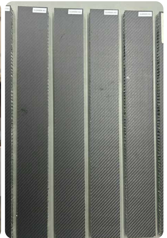
The test sample and setup for the long beam bending test to determine the bending stresses that the panel can withstand the core ribbons directions in the transverse and longitudinal direction. The tensile machine was used to compress the panel to cause it to bend and from which we could correlate our analytical results.
