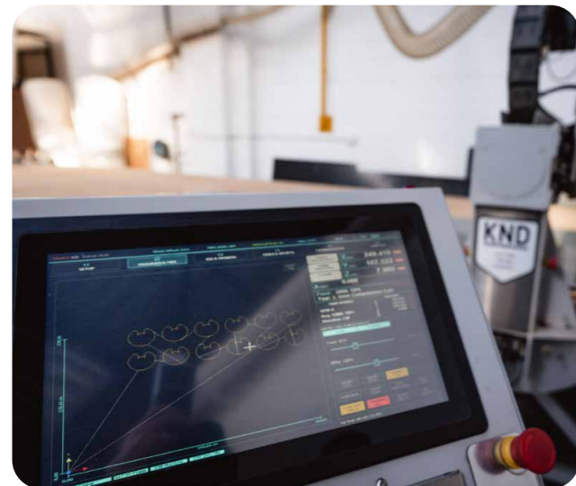
State of the art CAD and CNC cutting software used for designing and producing the components required for the boat production
