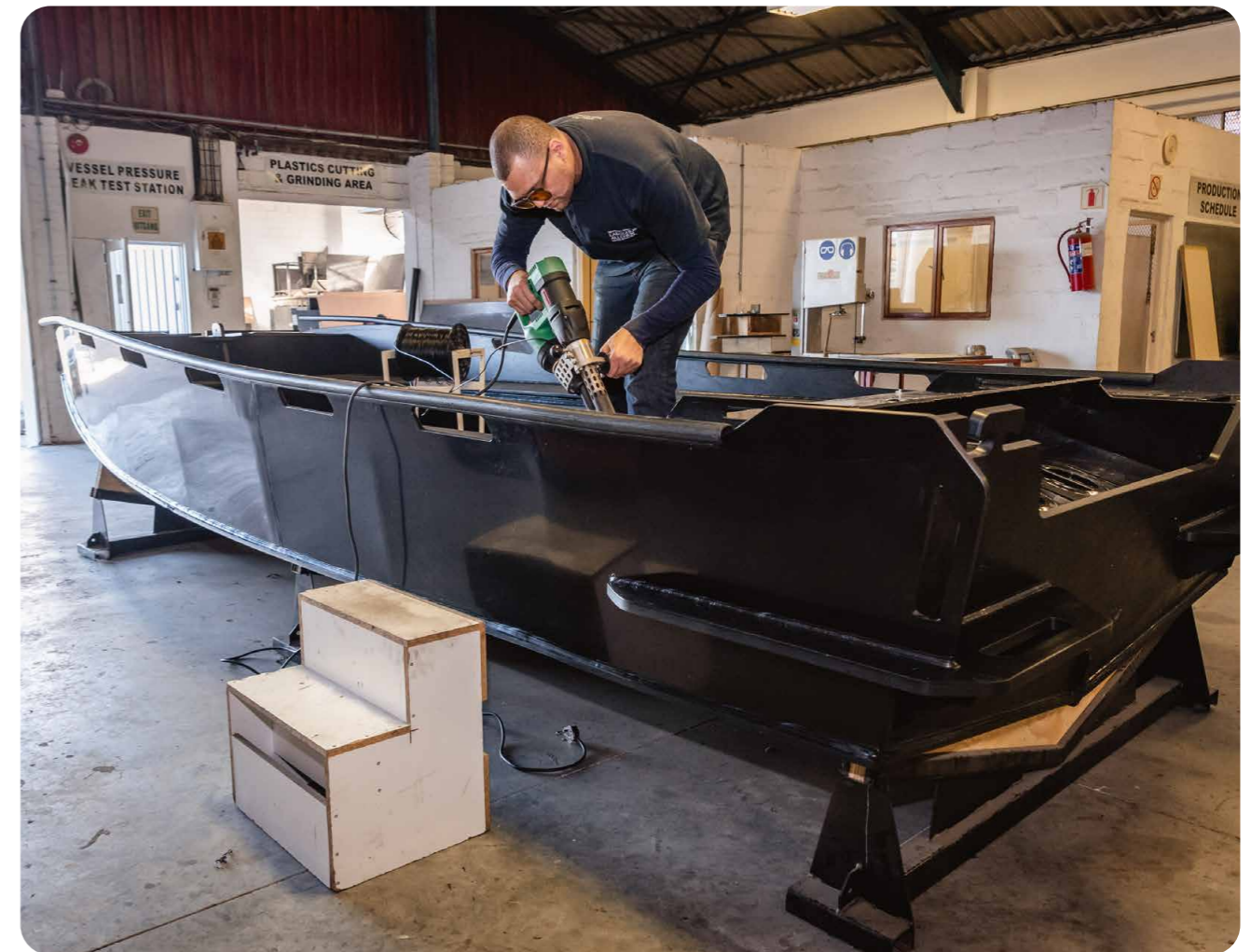
Nicolo Farmer, a senior fabricator and member of KND Fabrications, is seen here operating a plastic extrusion welder. This tool is essential for fusing HDPE plastic with a welding filament, ensuring strong and reliable joints in fabrications.
