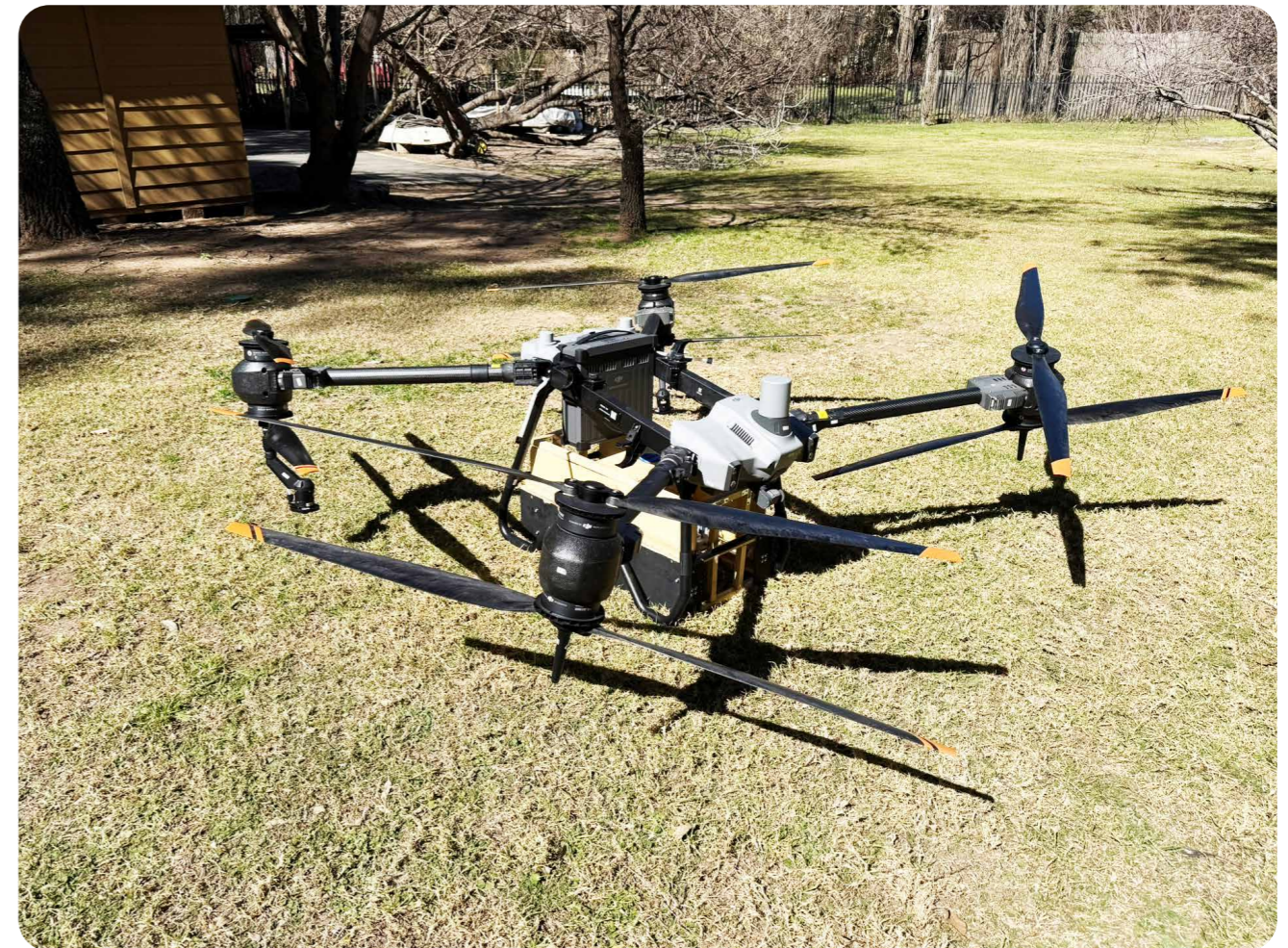
The drone utilised for this project is equipped with a coaxial twin rotor. The drone with eight motors in total (four coaxial pairs) is also known as an octocopter.
