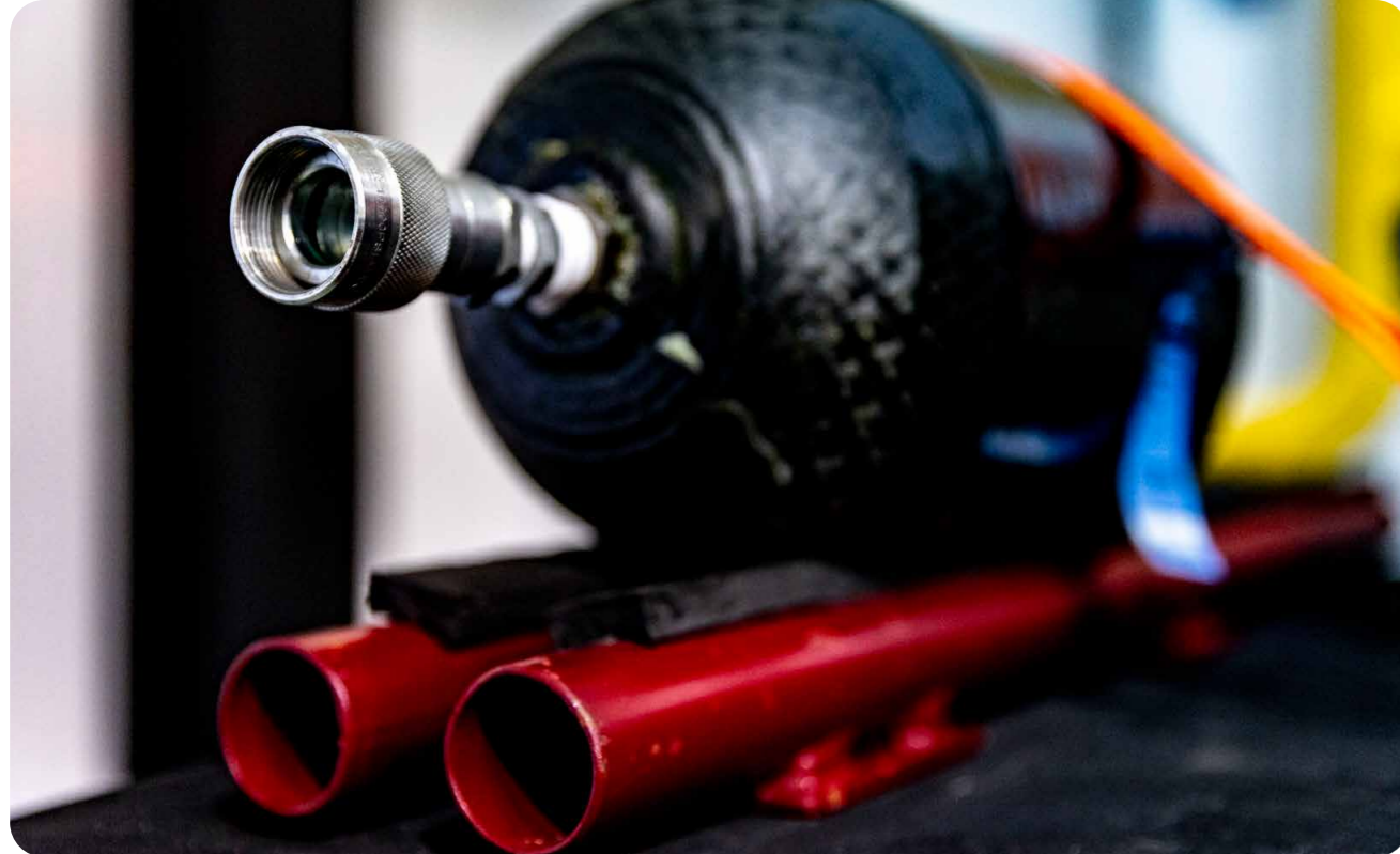
A Xenon tank produced by Petrawell attached to a hydrostatic test bench
