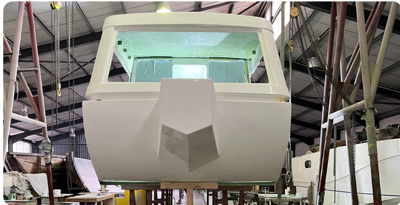
Side view of the first cabin produced from the mould
