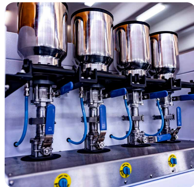
The raw material (metal powder) utilised for the 3D printing process is housed in a series of powder kegs.
