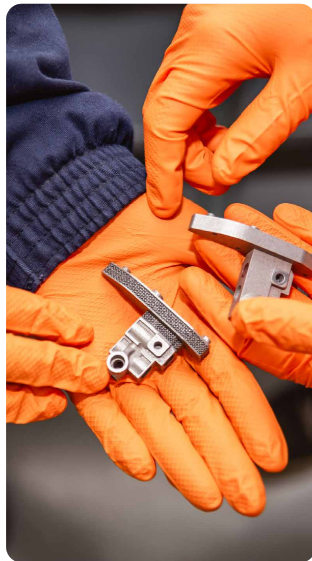
Additively Manufactured AlSi10Mg fuel manifolds evaluated for quality after post-processing comparing the two different designs for additive manufacturing (DfAM) iterations.
