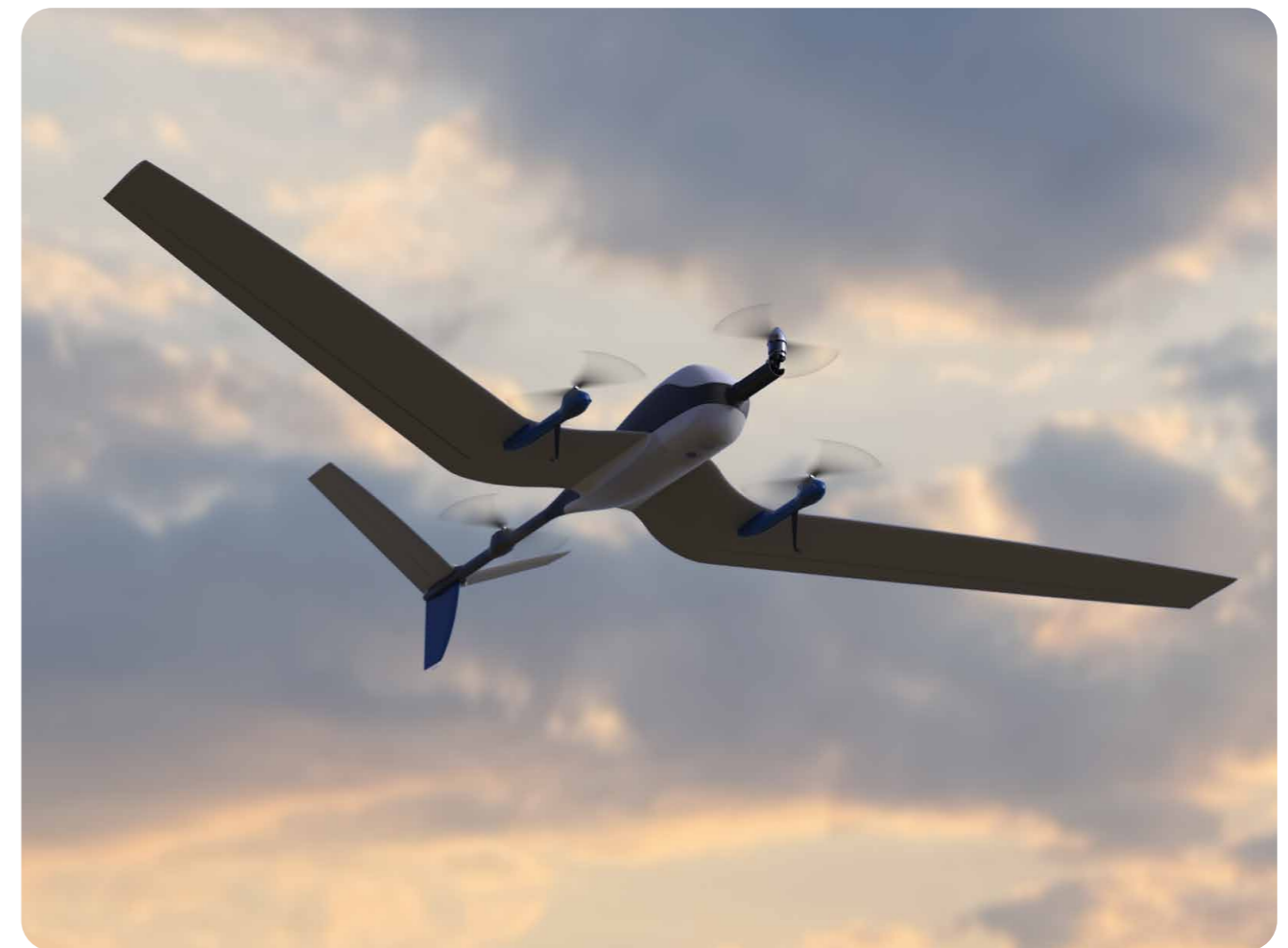
The Elevation is a small commercial vertical take-off and landing (VTOL) drone, redesigned with lightweight hybrid composites to reduce cost, weight, and production time while advancing toward industrialisation.
