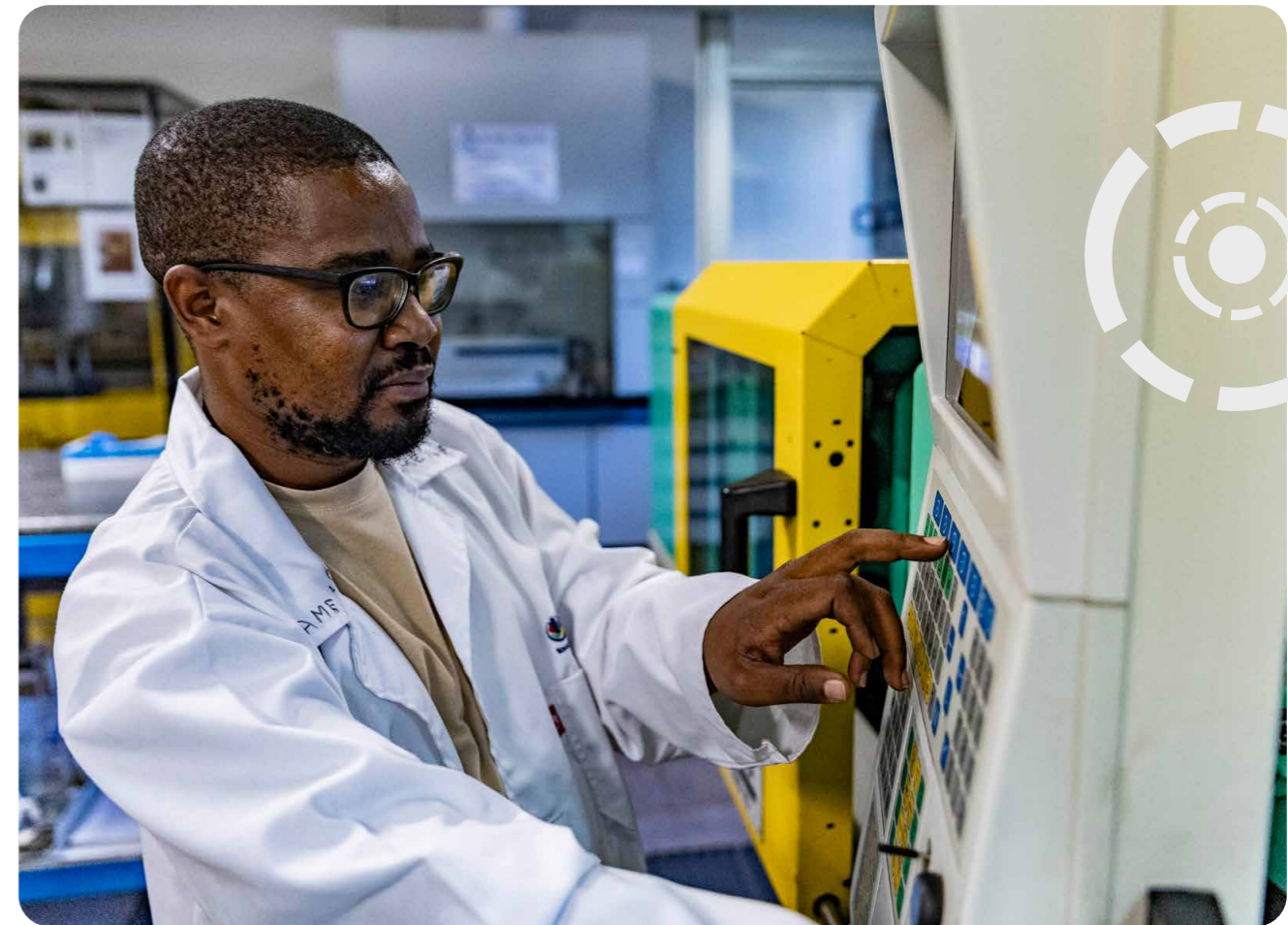
The CSIR's Mandy Madigoe, a Senior Engineer and Technical Leader on the project, is seen here preparing an Arburg MIM machine to produce green components.
