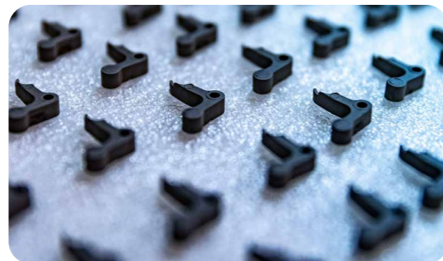
Prototype components produced through metal injection moulding (MIM) will advance South Africa's local capability to supply high-precision parts for the aerospace and defence sectors.
