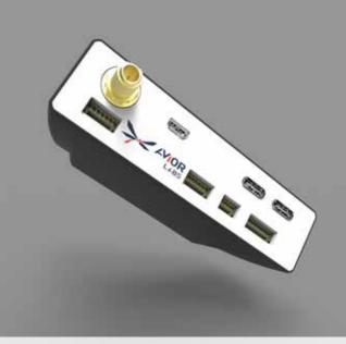
The housing is 3D printed from high strength nylon that offers a quality solution.
