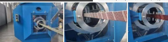
These images were taken of one of Wilec's first orders. For this particular order, netting tape was applied to the conductor bundle, which is usually at the request of the customer. The purpose of the netting tape is to improve oil flow and cooling in the final product (a transformer). The improved oil flow assists with improving the electrical performance of the transformer at the end user.
