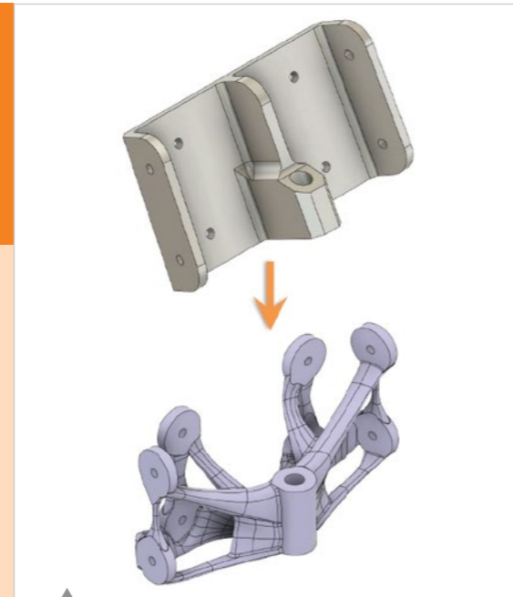
Original upper rudder hinge bracket design and topologically optimised design.
