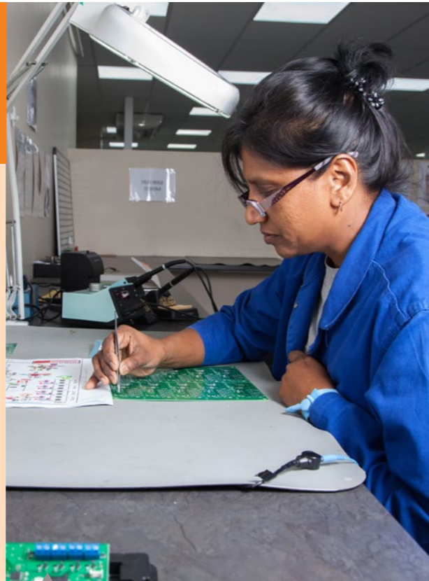
An experienced lab technician meticulously hand places a prototype PCB before reflow.
