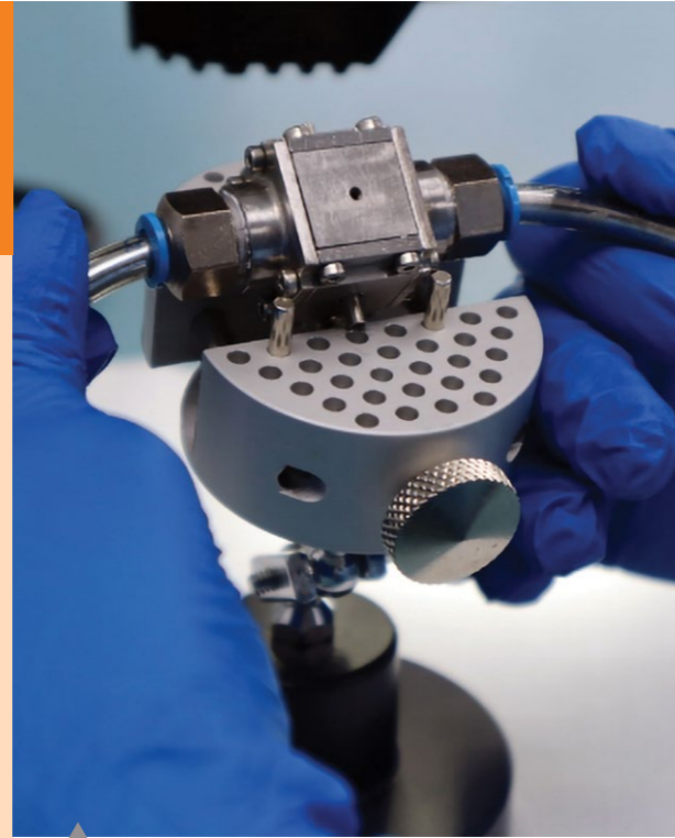
The single axis FLIA system designed to control a 1U cube satellite.
