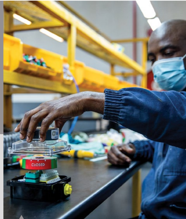
Assembling a valve position indicator.
