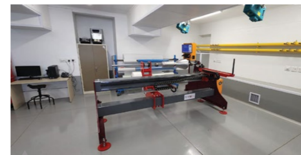
The filament winding facility produces composite vessels that address the storage and transportation needs of the aerospace and hydrogen market.
