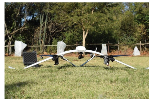
Bronberg Dynamics is providing the airframe for the project in the form of its COB vertical take-off and land UAV.
