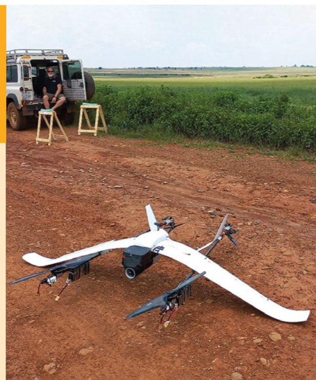
The novel hopper/counter (front centre of the airframe) integrated with the VTOL drone ready for take-off and testing.
