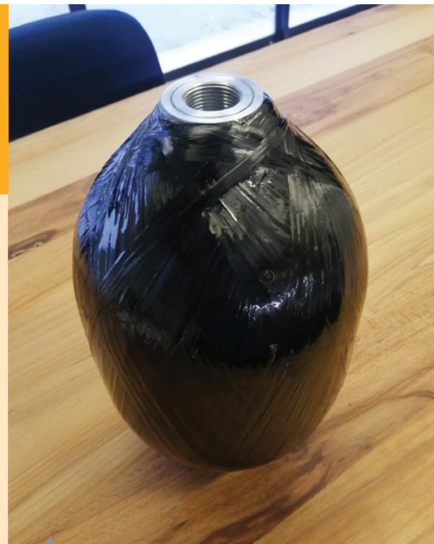
Close up of a vessel that has been wound with a composite filament.
