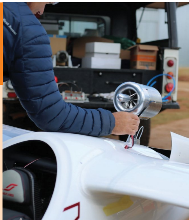
▲ CAT's 400 N turbojet is mounted on a Jonker Sailplane for testing.
