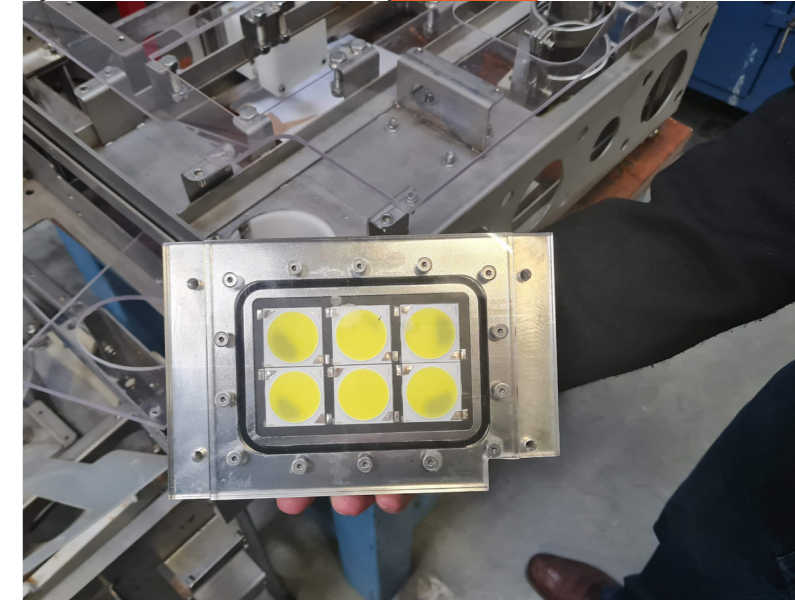
A custom payload frame design for LED lighting on an autonomous underwater vehicle, produced by Marine Solutions
