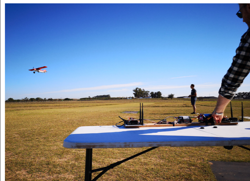
First field test of the Stereo Vision Approach Tracker using a scale model plane to collect data for processing and machine learning
