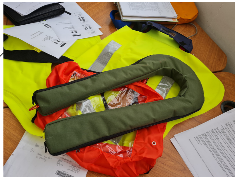
The Bladder (lime) and spray cover (orange), critical parts of the inflatable lifejackets manufactured by Zero° Industries
