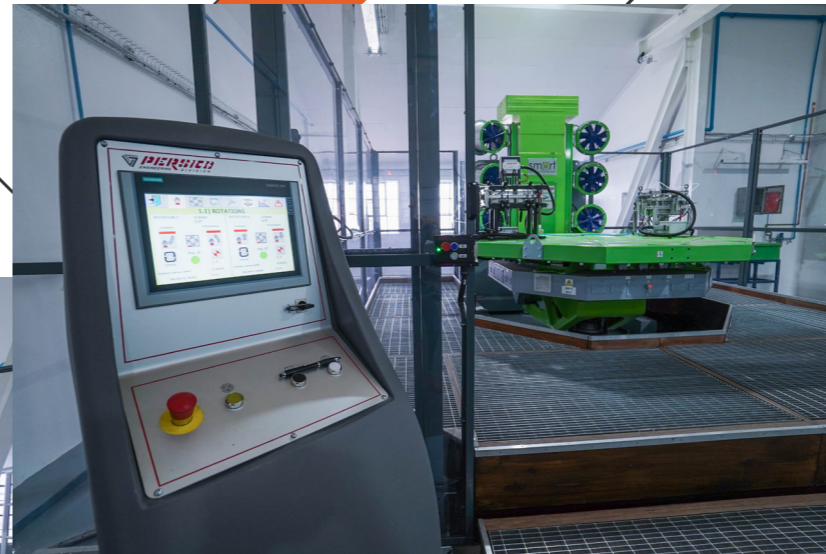
Precision control of processing parameters such as internal temperature, internal pressure, external cooling with direct heating technology
