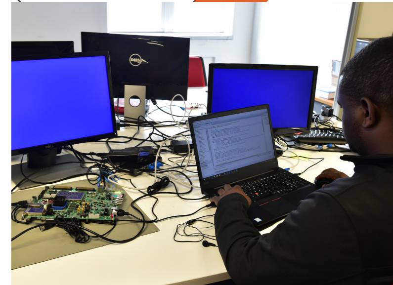
Development and Test environment for a Radio/Video processor to enable Long Range Unmanned(UAV)/Drone operations
