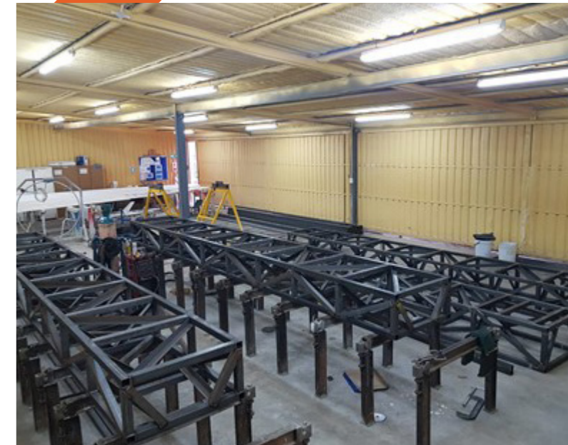
S5 Wing Mould Backing Structure
