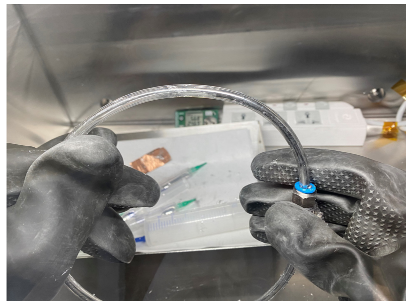
Fluid loop being filled in glovebox
