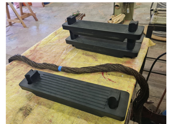
Rubber step and tarred twine used to whip the rope to the components
